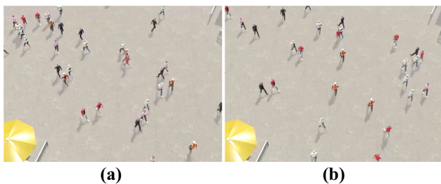
Fig. 8 The comparison between a the rendering of real-world crowd movements from ETH-Univ dataset, and b our simulation result with this dataset as input
